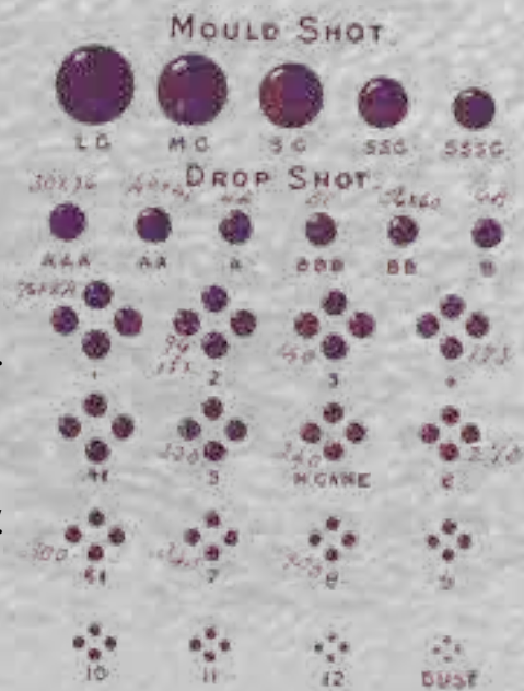
Diagram showing different sizes of lead shot made at Elswick.
